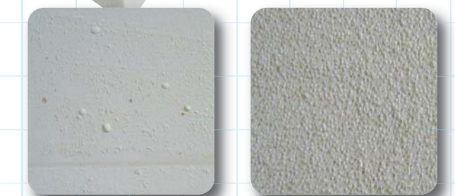
Microstructure Results (JM23 left) the carefully controlled micro porosity of JM23 IFB confers much improved thermal conductivity compared to the much larger pore size of Brand X bricks (the difference is easily seen in the photographs above).
